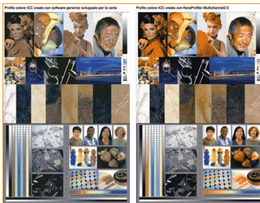
FIG. 9 - Comparison between an ICC colour profile created with general software developed for printing on paper (on the left) and an ICC colour profile created with Keraprofiler Multichannel 2.0
